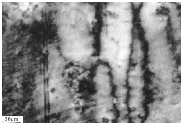
Figure 4. POM micrograph of an oriented film of polymer Pa (sheared at 140°C) and annealed at 140°C for 10 min.
